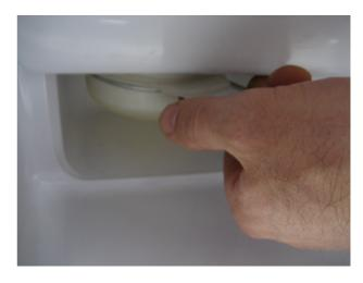
15. ....pour onto the evaporator cavity one or two liters of clean potable water with **cc 2 antibacteria solution** (part number 264000 02) to rinse and sanitize the molds and the spray system.
