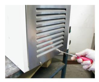
2. ....Top Panel to again access either to the control box and the evaporator.
