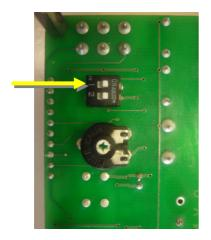
**First DIP SWITCH Key.** ON, standard position, supply power directly to the **Compressor**. OFF shuts-off the compressor. It replaces the previous Compressor Switch.
