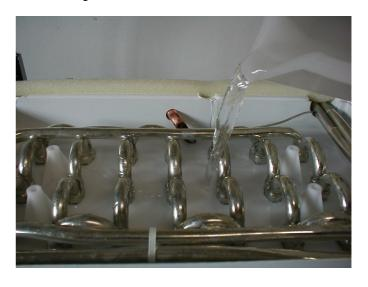
10. With help of a brush dissolve the most resistant and remote scale deposits in the platen.
